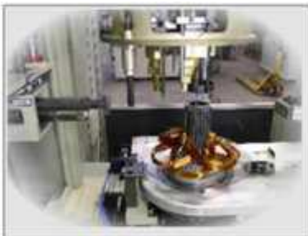
COIL WINDING UNIT
