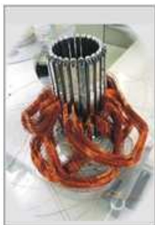
COIL INSERTING ZONE
